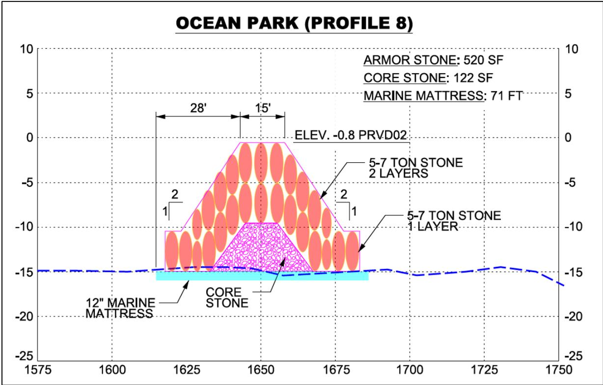
Figure A - 79. Cross-Section of Breakwaters in Eastern-Reach B
