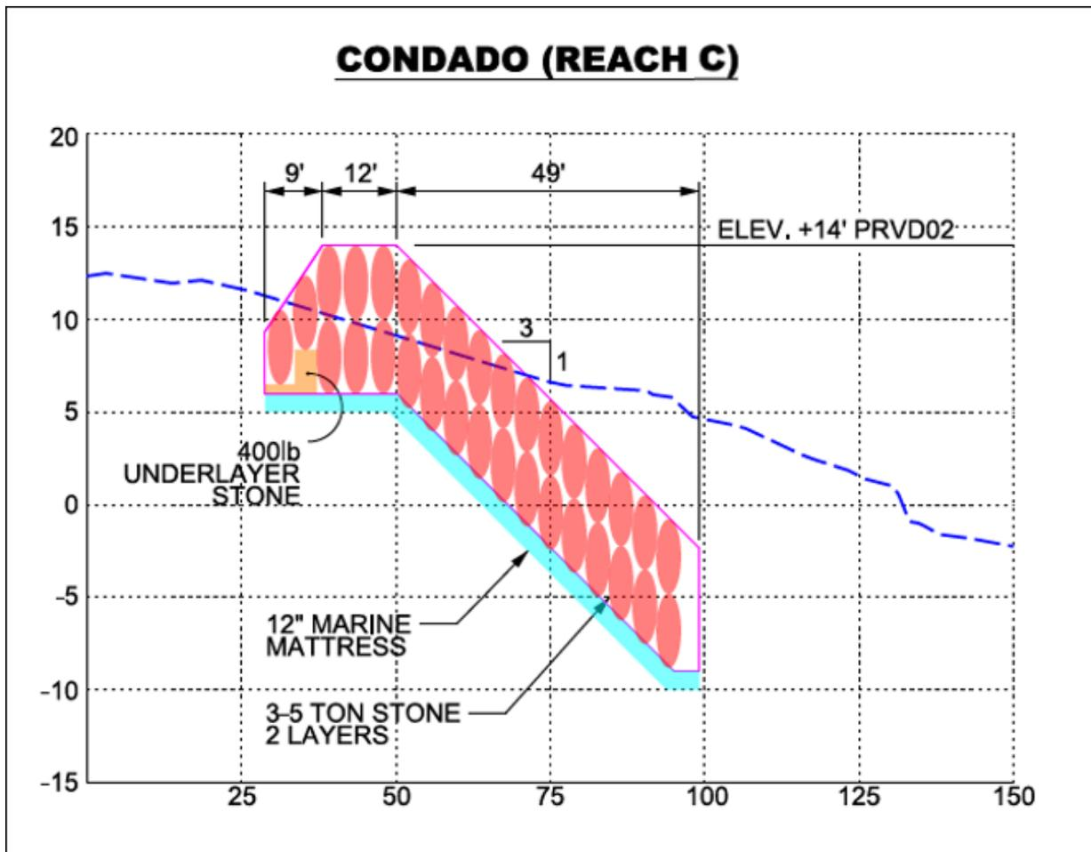
Figure A - 81. Condado's Reach C Revetment Design
