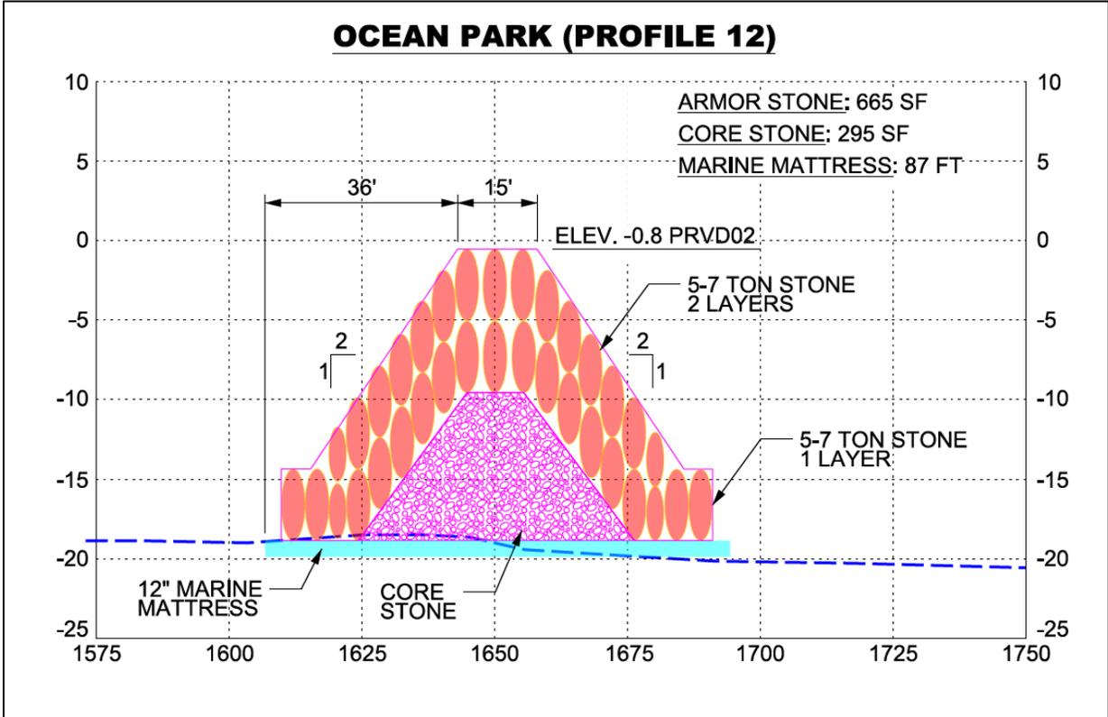
Figure A - 80. Cross-Section of Breakwaters in Western-Reach B
