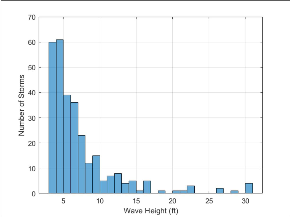
Figure A - 68. Distribution of Peak Wave Heights for OWI GFC-2 Grid Point 93294
