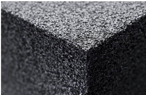
Closed-cell structure of FOAMGLAS® cellular glass insulation.
